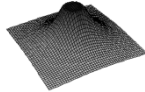
Three-dimensional simulation of the peak tissue temperature (at the time the pulse ends).
